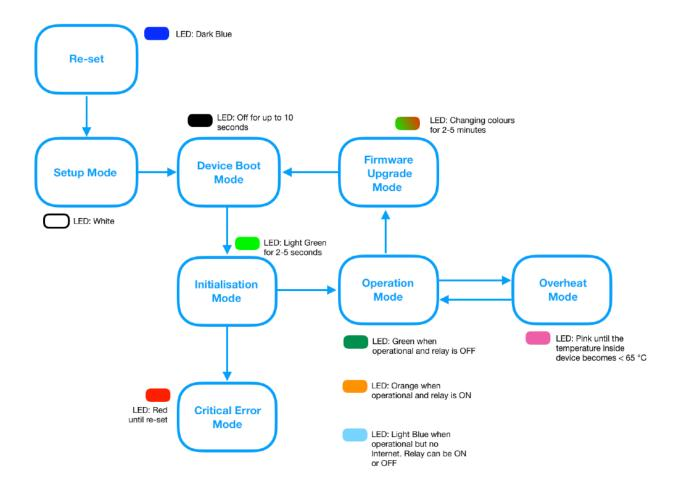
Please note that, that even though the device is in the Operation Mode and shows the correct LED status, the REST API may need up to 2 minutes to become fully accessible. Sending the /ping command via REST API after the device moves into the Operation Mode speeds up the process and makes the API accessible immediately.
